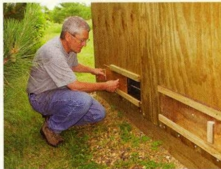
8 Vents allow moisture to escape during drying. They are closed toward the end of the drying process to help maximize heat and get the wood down to the target 8 percent MC.
