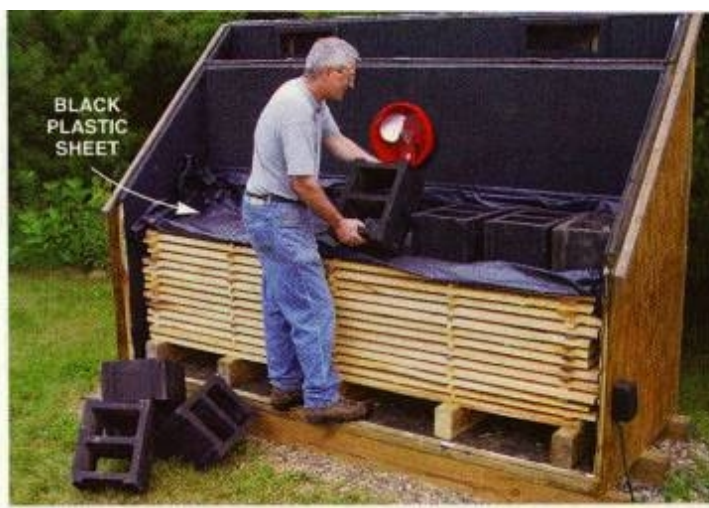
6 I topped the stack with cement blocks painted black for heat absorption. The weight from the blocks reduces warping in the drying wood. A plastic sheet attached to the plenum and draped over the top of the stack forces air through the stack.
