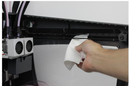
9. Clean the guides with the solvent pencil, making sure that it does not drip with special emphasis on the superior and inferior faces.
