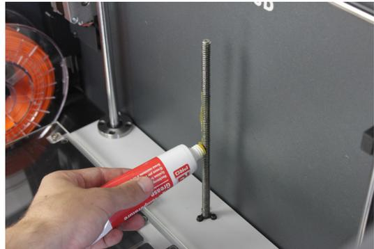
6. Turn on the Sigma and from the LCD screen, go to *Utilities --> Maintenance--> Move printing surface*. Raise and lower the platform twice to evenly distribute the oil and grease. Finally, remove the remnant grease.
