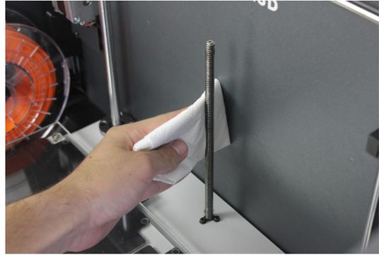
5. Apply the grease along the spindle of the Z-axis motor.
